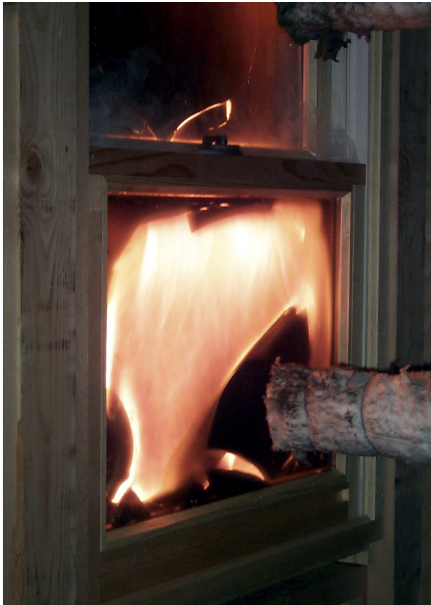
Figure 16. The flame contact exposure during laboratory testing of this wood-frame, dual-pane window resulted in glass breakage. The relatively large pieces of glass that remain indicate that annealed glass was used. Photo: Stephen L. Quarles.
